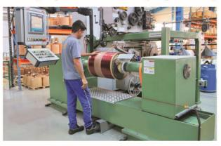
Drying process is done on all windings and act as a key role to guarantee safety and reliability of winding during the life cycle.
